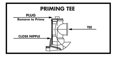
Suction pipe should be at least  $1\frac{1}{2}$ "; a larger size may be used if horizontal runs are required in addition to the vertical drop pipe. Priming will be facilitated if a tee or cross is used at the pump discharge with a priming plug on top.
